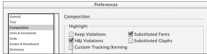
FIGURE 4-52 Highlighting Loose and Tight Lines
