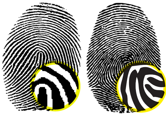
Figure 5. The fingerprint on the left is a raster image, the fingerprint on the right is a vector image.
